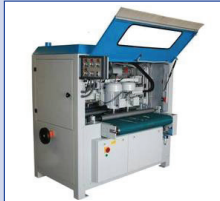
Model DiscMaster 4TD Abrasive disc deburrer. For one sided deburring only.
