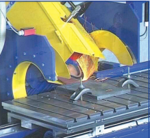
Model KMU Abrasive belt edge bevelling machine.
