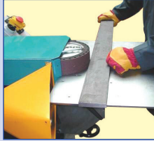
Manual de-slagging with special design belt grinder.
