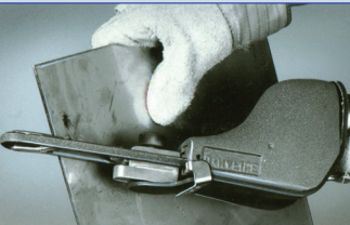
For the occasional sheet deburring, consider using a portable abrasive power tool with a special cranked arm.
