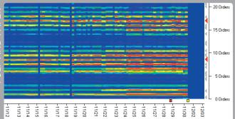
The **Colored Spectrum Overview** from a twin wire press verifies that the signal origins from the inner race. The twin wire press runs at 10 to 15 rpm. The patterns consist of the center frequency with sidebands. After the replacement, marked with a yellow square, the bearing signals completely disappear.
