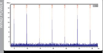
The **Spectrum** from a main shaft bearing on a wind turbine, NM52 900 kW, shows a damage on the outer ring. The shock pulse level is still very low but the spectrum is showing a developing damage. The shaft is rotating at 22 rpm. The wind turbine generated 752 kW, which is 84% of full effect.
