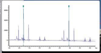
The **Time Signal** from a steel bar mill gearbox shows a broken roller. The bearing is running at 64 rpm. The time between the markers corresponds to the rpm of the rollers. The time domain is a very powerful tool when doing in depth analysis of the running condition of a machine.
