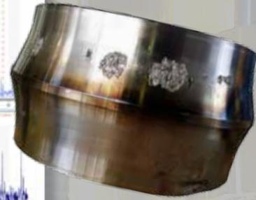
A clear spall on an inner race detected by HD technology in a ball mill application.
