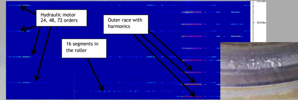
In the above Color Spectrum Overview, there are a number of distinct horizontal lines related to what is know as the commutation frequency from the hydraulic motor at 24, 48, 72, 96 orders. The outer race bearing signals are also clearly identified in the above plot.
