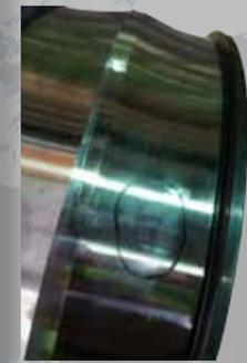
A Color Spectrum Overview from a gearbox driving a mine cage. The development of this clear inner race spall was monitored for six months prior to replacement.
